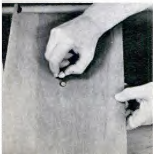
SCREWS are hidden by turned buttons, or you can use dowel ends cut to fit and then sanded flush
